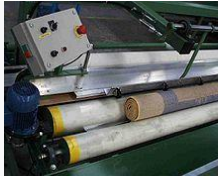
Machine used to cut and re-roll carpet lengths
